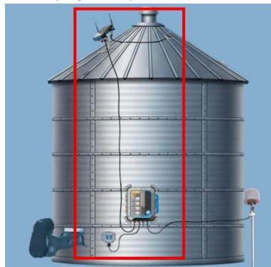
Figure 3: Example Connection Between EPIQ+ Fan Node and EPIQ Cable Node Shown
