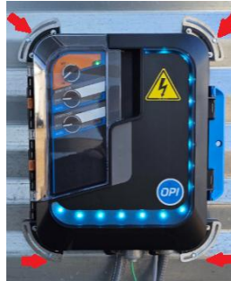
Figure 2: Mounting Screw Locations on EPIQ+ Fan Node
