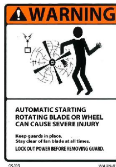
Figure 23 Caution Fan Warning Sticker
