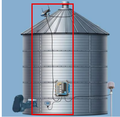
Figure 12: Overview of Plenum Sensor Installation
