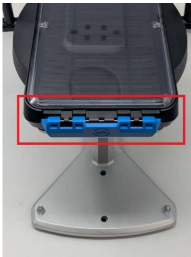
Figure 7. Closed Node Showing Secure Clasp
