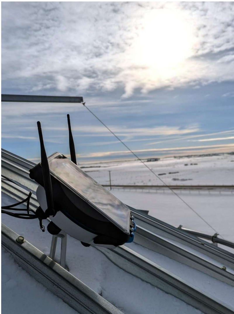
Figure 4. Node installed on Bin Roof
