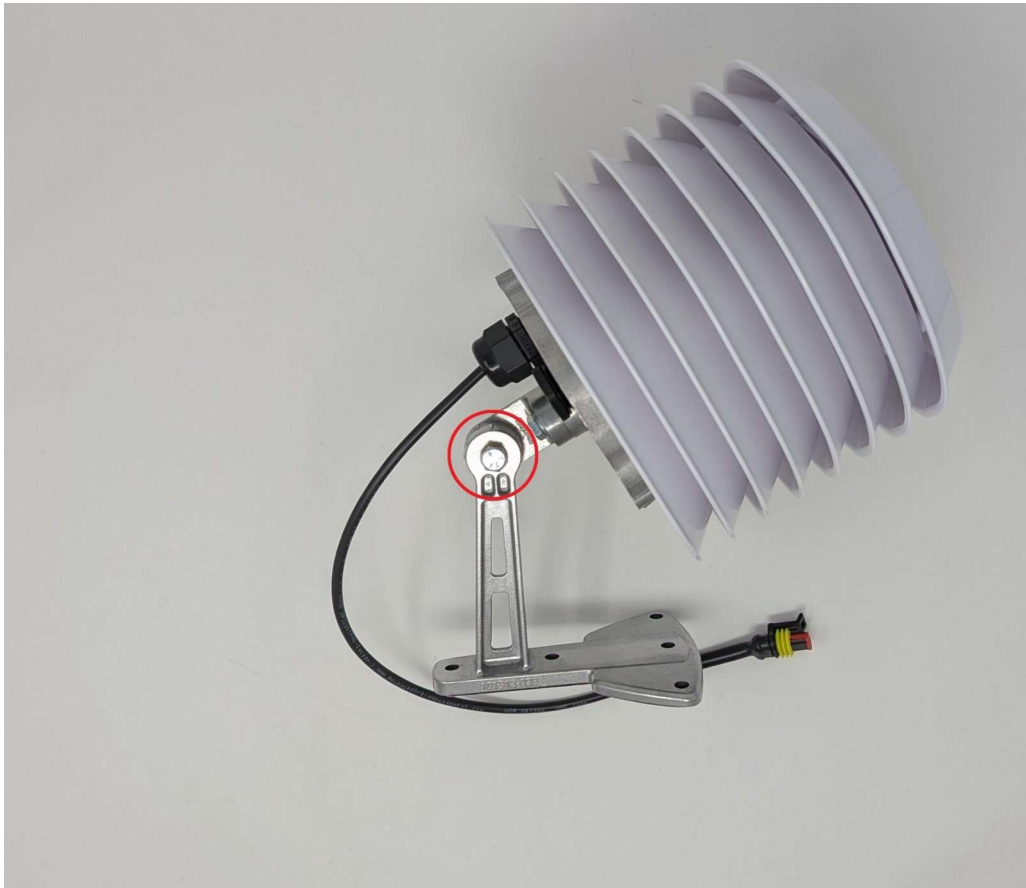
Figure 3. Foot Mount Adjustment Bolt
