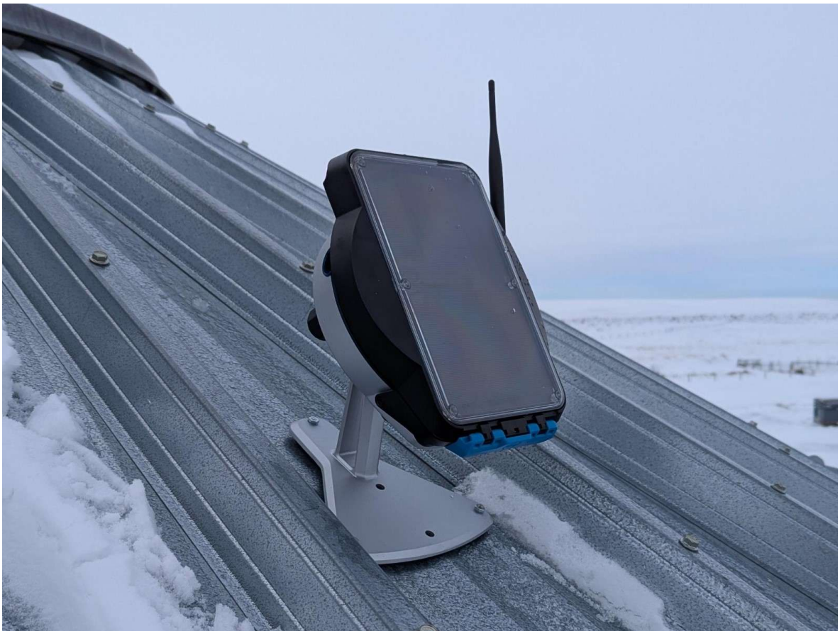
Figure 4. Node installed on Bin Roof
