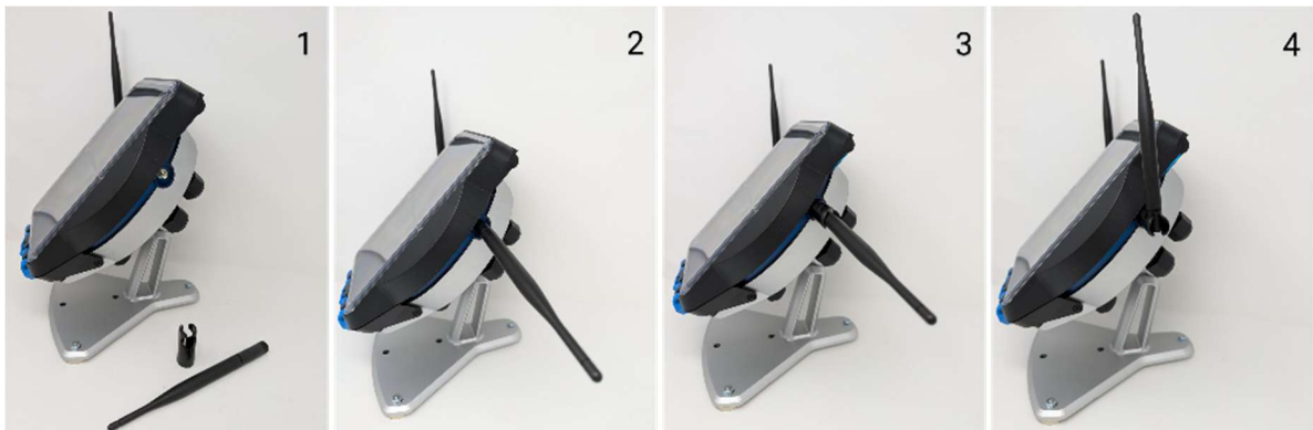
Figure 7. Antenna Locking Procedure
