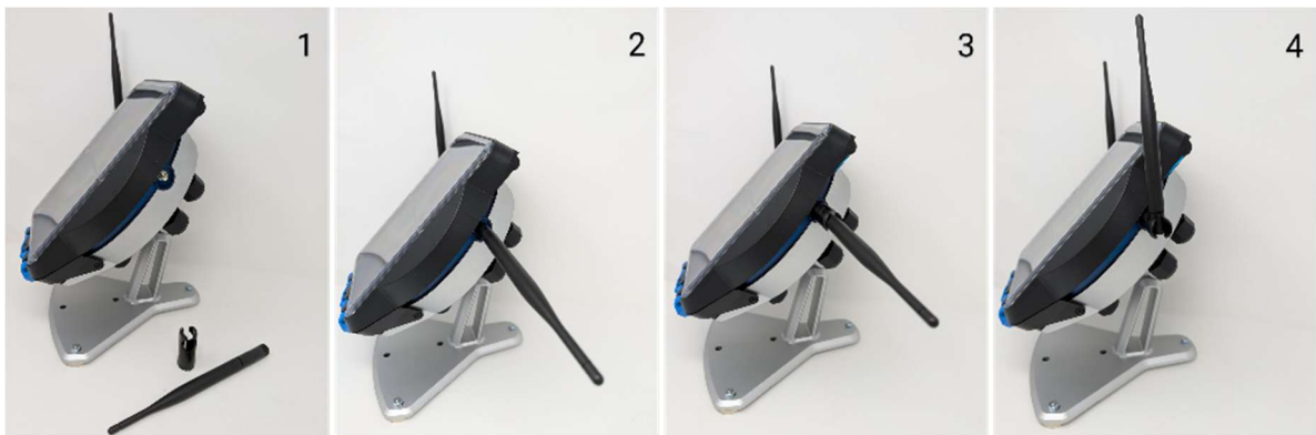
Figure 7. Antenna Locking Procedure
